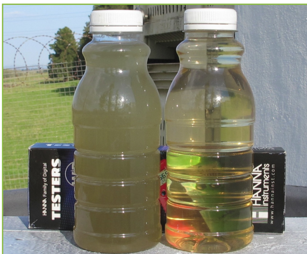
Samples. After inert solids interceptor on left and after SOG filter
